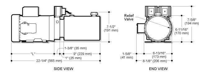
"L" dimension shown for 08751 motor is 10-11/16" (271 mm) Dimensions will vary according to motor output and manufacturer
