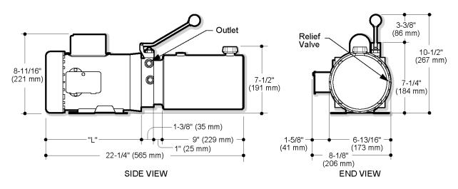
"L" dimension shown for 08751 motor is 10-11/16" (271 mm) Dimensions will vary according to motor output and manufacturer
