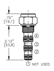
PORT #3 (INLET) IS ONE SIZE LARGER THAN PORTS #2 & #4 (OUTLET). FOR ALUMINUM OR STEEL VALVE HOUSING CONFIGURATIONS SEE PAGE 0-041.2
